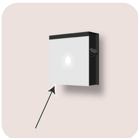
Image 4: Position of the identification label
